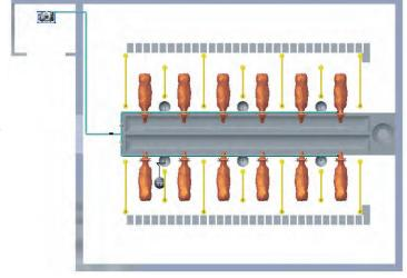
Figure: 2.2: (b) Milking Machine Installation Schematic in cow shed-Plan
