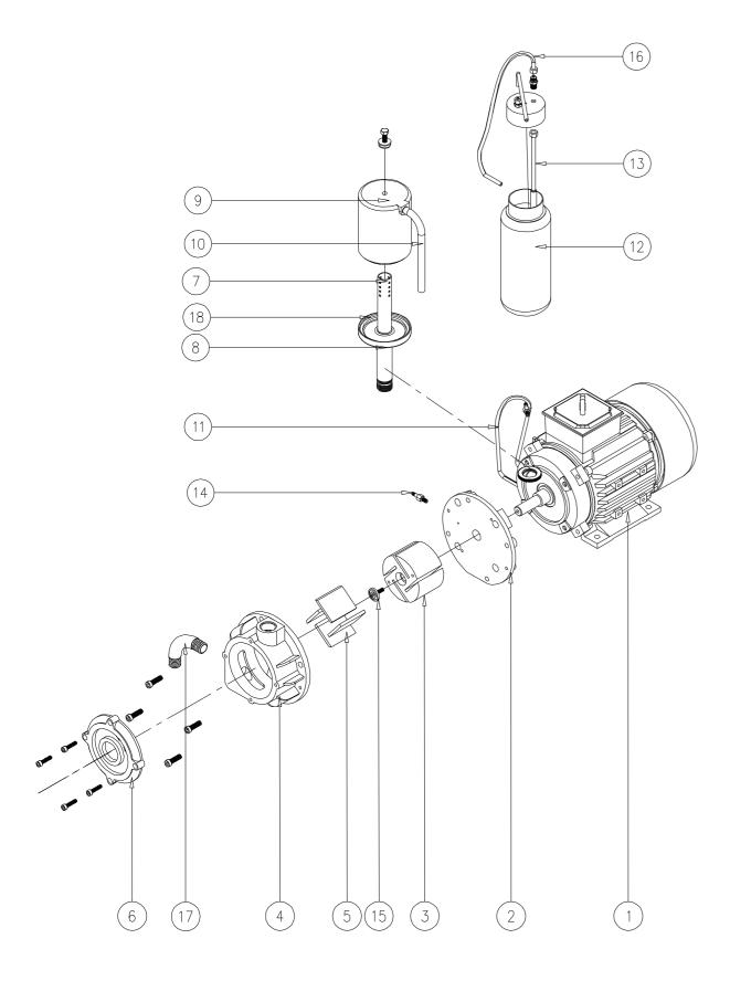
Figure 9.7 VAPA2000C0000000000 VACUUM PUMP
