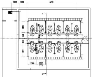
Figure: 2.2: (a) Milking Machine Installation Schematic in cow shed-with dimensions
