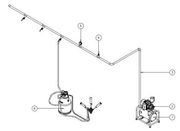
Figure: 2.1: Milking Machine Installation
