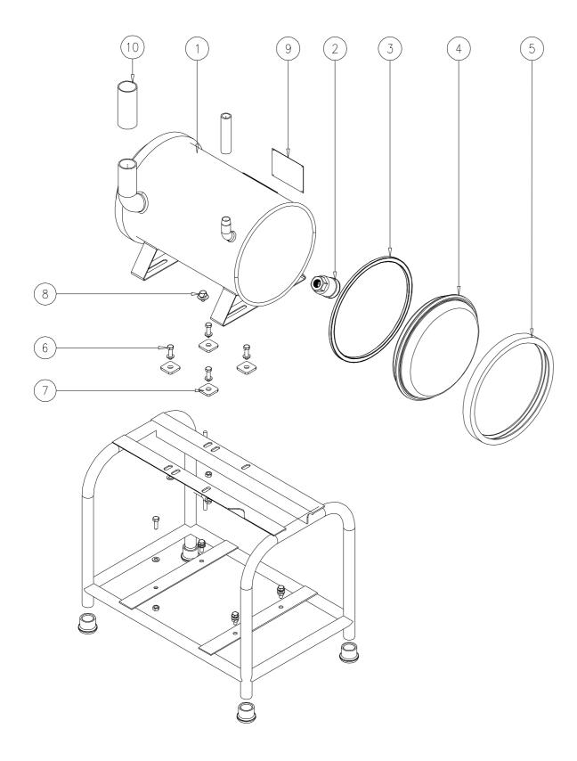
Figure 9.2 MLA0A00000000000000 VACUUM RECEIVER TANK
