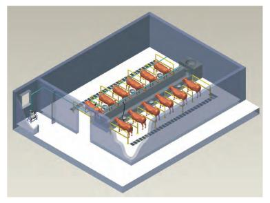
Figure: 2.2 (C) Milking Machine Installation Schematic in cow shed-isometric view
