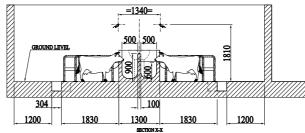
Figure: 2.2: (d) Milking Machine Installation Schematic in cow shed-sectional view
