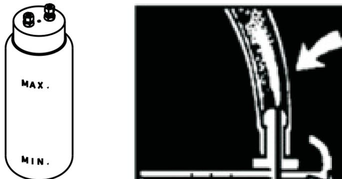
Figure No:2.3: Minimum and maximum levels in the oil bottle.
